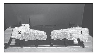
**STEP 3:** (SRV2057-721): Place log 2, nose to nose with log 1. The bottom notch on log #2 must mate over the log tab on the burner face.
